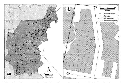
Figure 5. (a) Geocoded points (black dots) that are in a different CD (white bordered regions) to their cadastral centroid. (b) Displacement from the corresponding centroid CD due to line simplification in the CD boundary file. A small increase in the geocoding offset would be sufficient to place the geocoded points into the correct CD.
