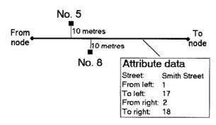
Figure 1. Example geocode line segment with an offset of 10 m (inset not shown).
