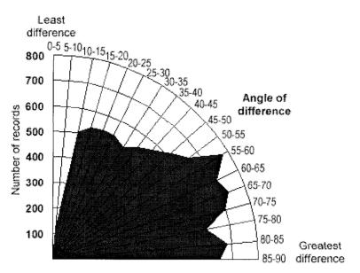
Figure 4. Quadrant radar diagram indicating the degree of difference between a line perpendicular to a geocode street segment and the line between the geocoded point and the concordant cadastral centroid.
