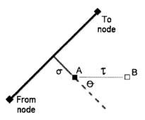
Figure 3. Line segment from a standard TIGER-type geocode file with an offset to geocoded location A. The centroid for the cadastre polygon is shown as B and the angle  $\theta$  indicates the amount of variation from the perpendicular.
